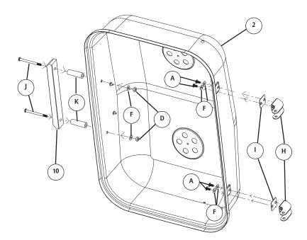
**Note:** Attach both ends of lid handle before fully tightening hex flange nuts.
